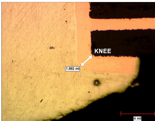
Figure 6. Cu Thickness Measurement Locations
